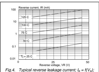
Fig.4. Typical reverse leakage current;  $I_R = f(V_R)$ ; parameter  $T_i$
