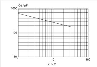
Fig.5. Typical junction capacitance;  $C_d = f(V_R)$ ; f = 1 MHz;  $T_j = 25^{\circ}$ C to 125  $^{\circ}$ C.
