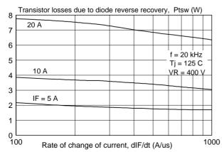
Fig.5. Typical switching losses in transistor due to reverse recovery of diode, as a function of of change of current dl /dt.
