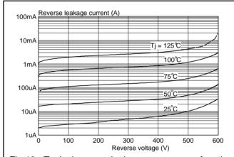
Fig.13. Typical reverse leakage current as a function of reverse voltage.  $I_R = f(V_R)$ ; parameter  $T_i$
