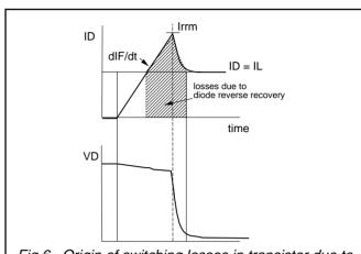
Fig.6. Origin of switching losses in transistor due to diode reverse recovery.
