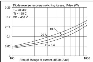
Fig.4. Typical reverse recovery switching losses in diode, as a function of rate of change of current dl<sub>e</sub>/dt.
