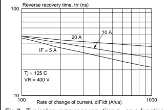
Fig.7. Typical reverse recovery time t<sub>rr</sub>, as a function of rate of change of current dl<sub>r</sub>/dt.
