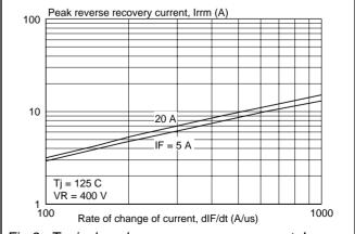
Fig.8. Typical peak reverse recovery current, I<sub>rm</sub> as a function of rate of change of current dI<sub>r</sub>/dt.
