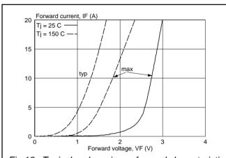
Fig.12. Typical and maximum forward characteristic  $I_F = f(V_F)$ ;  $T_i = 25^{\circ}C$  and  $150^{\circ}C$ .
