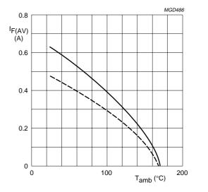
$$\begin{split} &V_R = V_{RRMmax}, \, \delta = 0.5; \, a = 1.57. \\ &\text{Device mounted as shown in Fig.7;} \\ &\text{solid line: Al}_2O_3 \, PCB; \, dotted line: epoxy PCB. \end{split}$$
