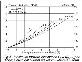
Fig.4. Maximum forward dissipation  $P_F = f(I_{F(AV)})$  per diode; sinusoidal current waveform where a = f orm f actor  $= I_{F(RMS)} / I_{F(AV)}$ .
