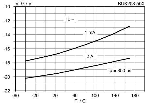
Fig.28. Typical negative load clamping voltage.
