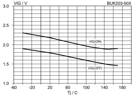
Fig.16. Typical input threshold voltages.
