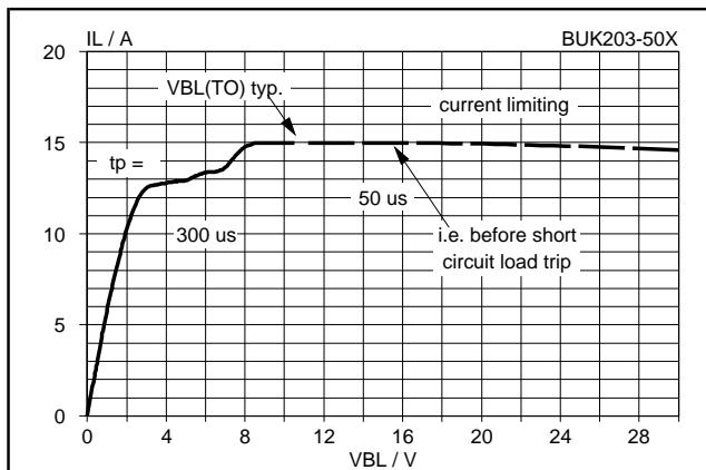
Fig.33. Typical overload characteristic,  $T_{mb} = 25^\circ\text{C}$ .
