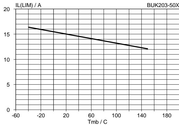
Fig.34. Typical overload current,  $V_{BL} = 9\text{ V}$ .
