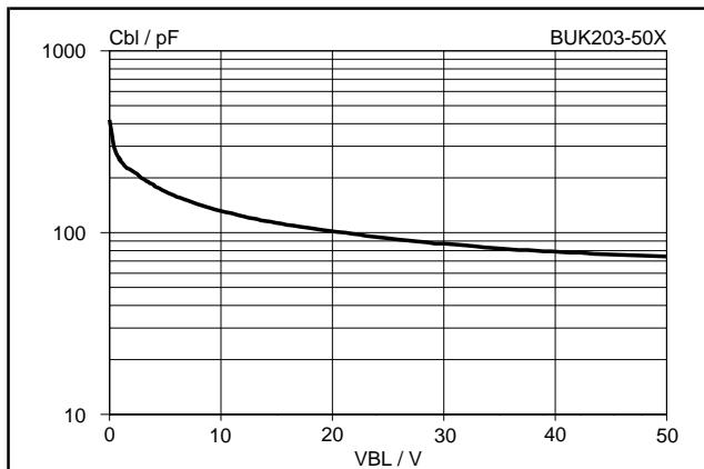
Fig.32. Typical output capacitance.  $T_{mb} = 25^\circ\text{C}$
