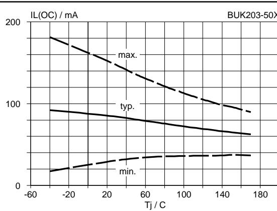
Fig.23. Low load current detection threshold.
