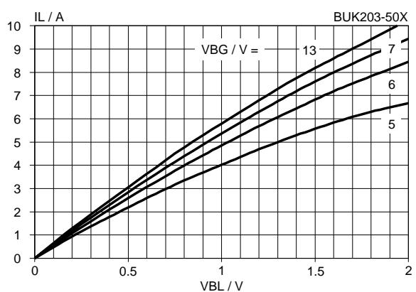
Fig.7. Typical on-state characteristics,  $T_j = 25^\circ\text{C}$ .
