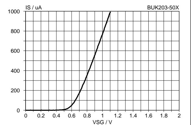
Fig.20. Typical status low characteristic,  $T_j = 25^\circ C$ .
