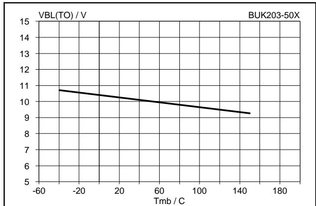
Fig.36. Typical short circuit load threshold voltage.
