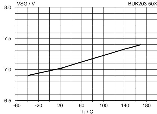
Fig.22. Typical status clamping voltage,  $V_{SG} = f(T_j)$ .
