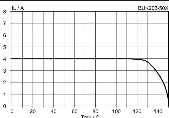
Fig.6. Limiting continuous on-state load current.
