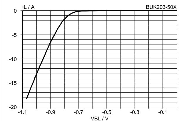
Fig.31. Typical reverse diode characteristic.
