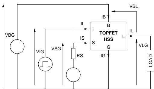
Fig.4. High side switch measurements schematic.
