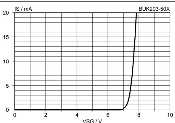
Fig.18. Typical status characteristic,  $T_j = 25^\circ C$ .
