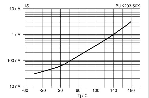
Fig.19. Typical status leakage current.
