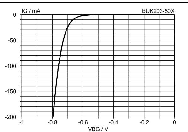
Fig.30. Typical reverse battery characteristic.
