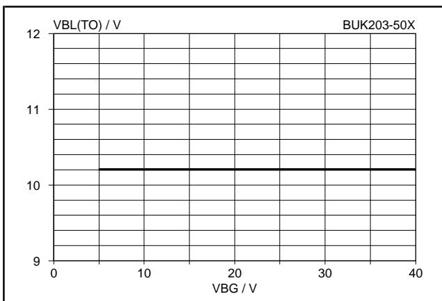
Fig.35. Typical short circuit load threshold voltage.
