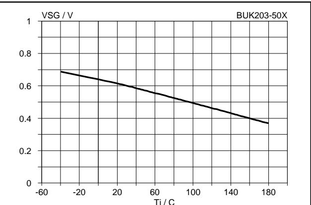
Fig.21. Typical status low voltage,  $V_{SG} = f(T_j)$ .
