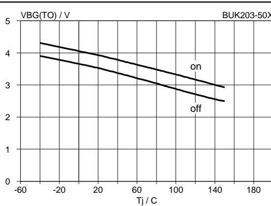
Fig.24. Supply typical undervoltage thresholds.
