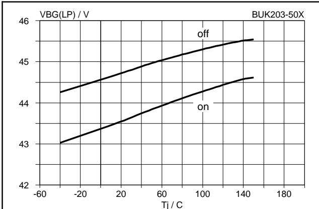
Fig.25. Supply typical overvoltage thresholds.
