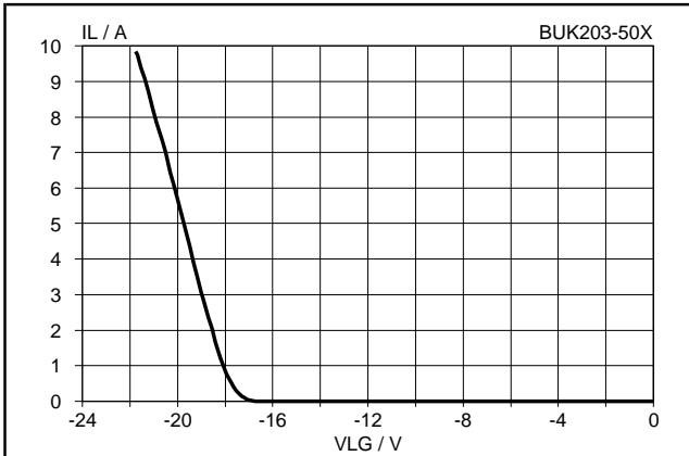
Fig.27. Typical negative load clamping characteristic.
