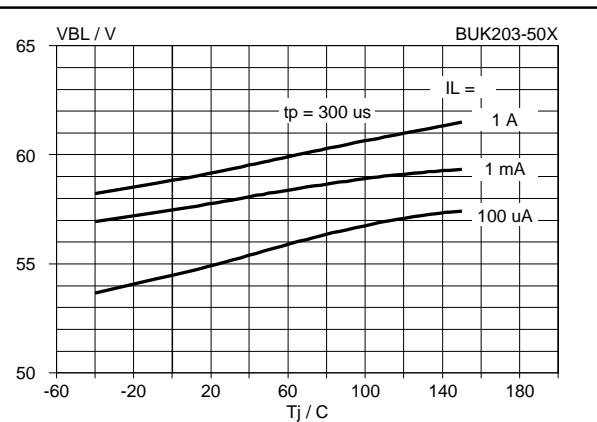
Fig.29. Typical battery to load clamping voltage.
