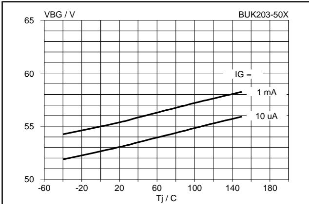
Fig.26. Typical battery to ground clamping voltage.
