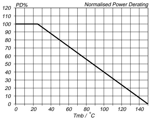
Fig.5. Normalised limiting power dissipation.
