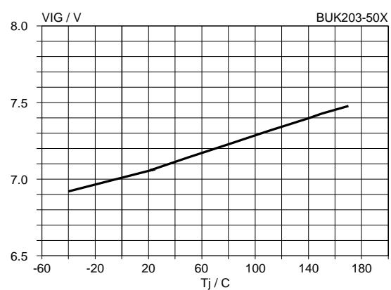
Fig.17. Typical input clamping voltage.
