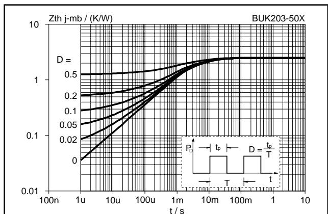
Fig.37. Transient thermal impedance.
