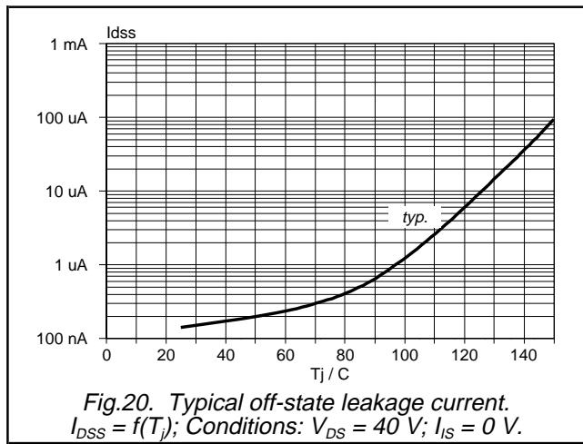
Fig.20. Typical off-state leakage current.
