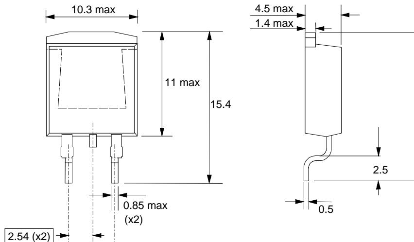
Fig.22. SOT404 : centre pin connected to mounting base.
