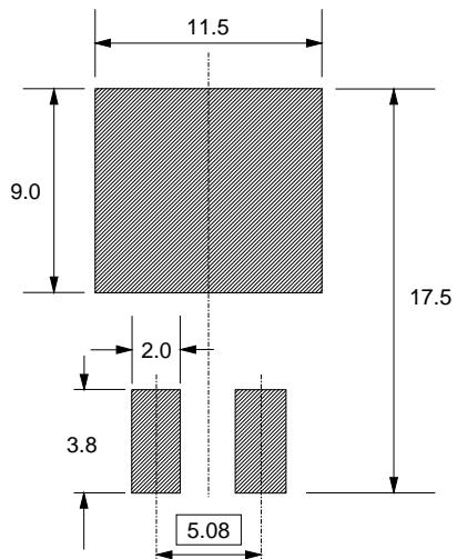
Fig.23. SOT404 : minimum pad sizes for surface mounting.
