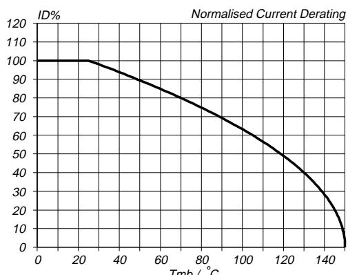
Fig.3. Normalised continuous drain current.
