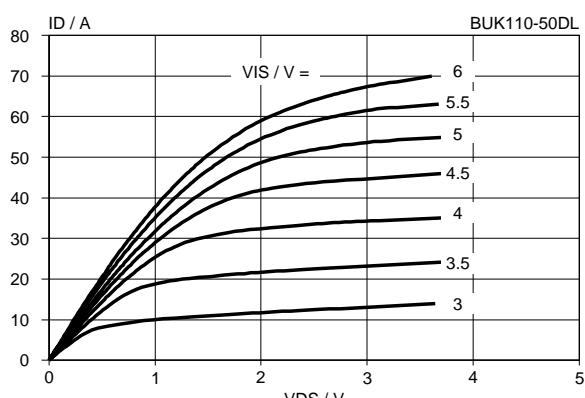
Fig.6. Typical on-state characteristics,  $T_j = 25^\circ C$ .
