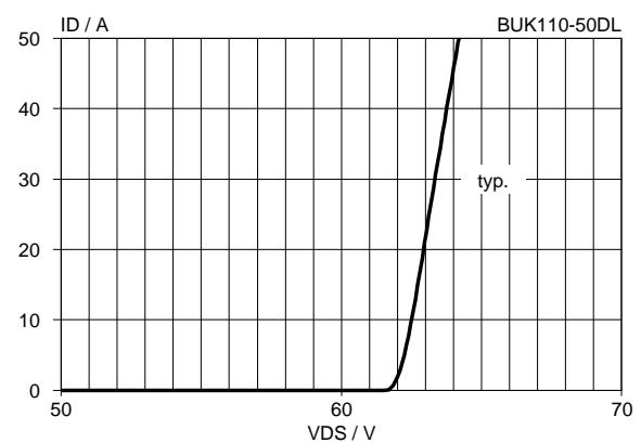
Fig.12. Typical clamping characteristics,  $25\text{ }^\circ\text{C}$ .
