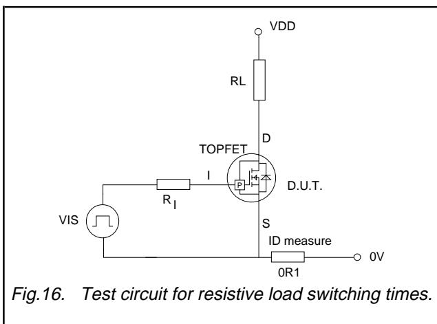
Fig. 16. Test circuit for resistive load switching times.
