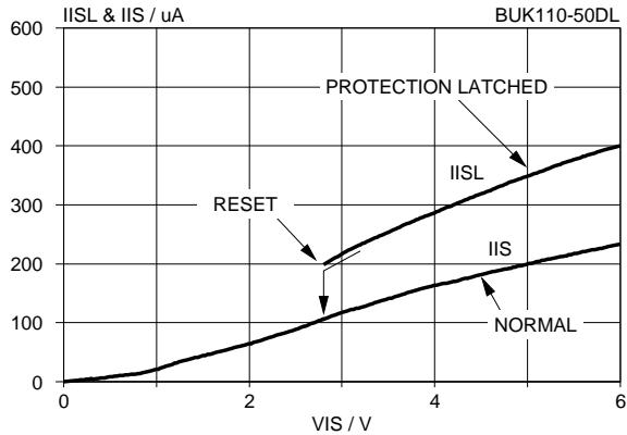
Fig. 14. Typical DC input characteristics,  $T_j = 25^\circ\text{C}$ .
