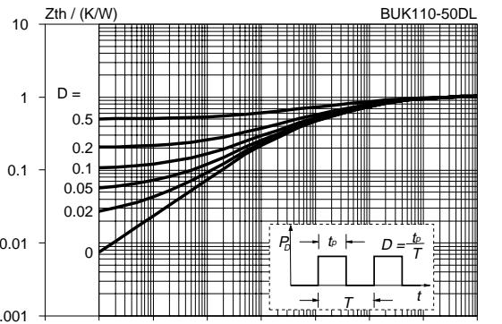
Fig.5. Transient thermal impedance.
