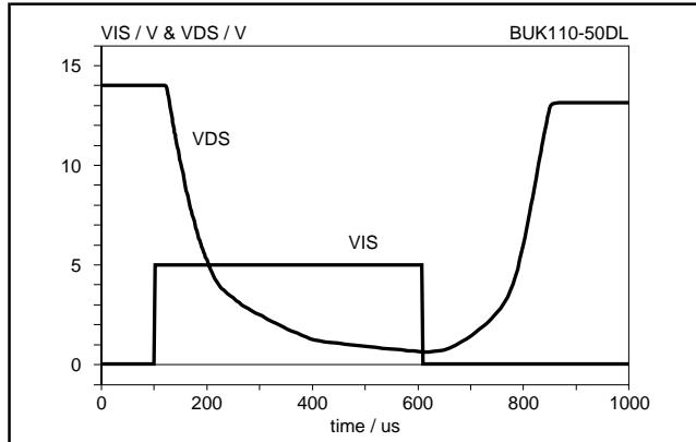
Fig. 17. Typical switching waveforms, resistive load.
