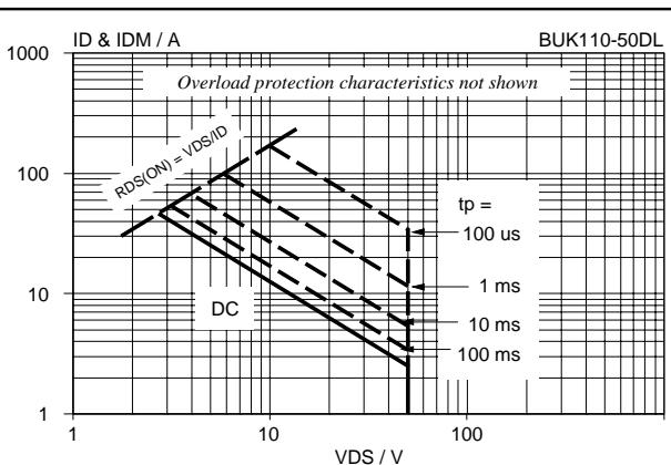
Fig.4. Safe operating area.  $T_{mb} = 25^\circ C$
