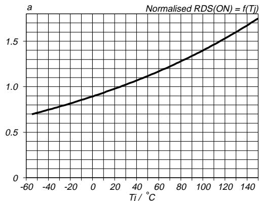
Fig.8. Normalised drain-source on-state resistance.
