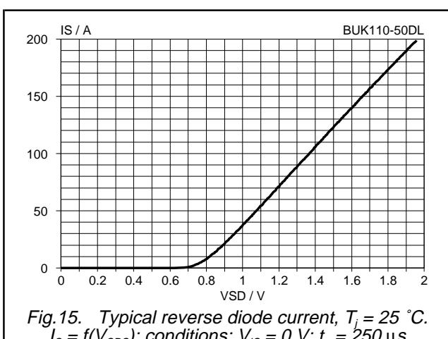
Fig. 15. Typical reverse diode current,  $T_j = 25^\circ\text{C}$ .
