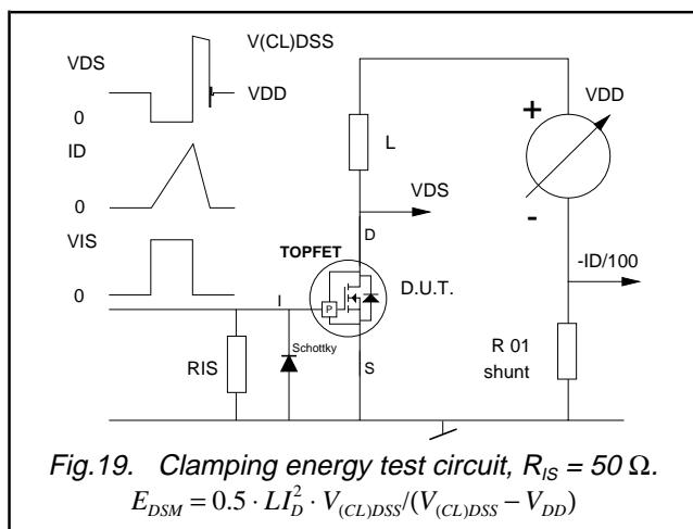
Fig. 19. Clamping energy test circuit,  $R_{IS} = 50\Omega$ .
