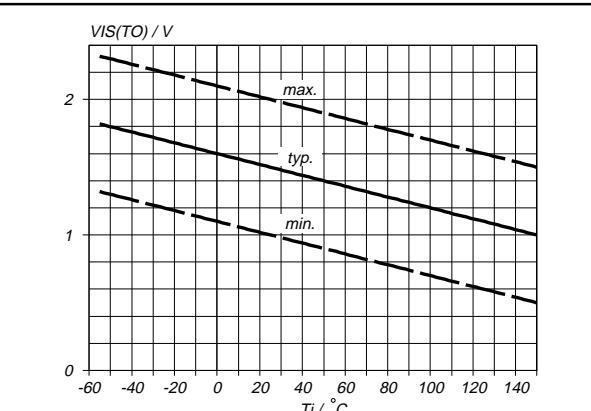
Fig.13. Input threshold voltage.
