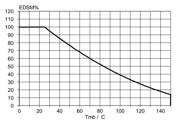
Fig. 18. Normalised limiting clamping energy.
