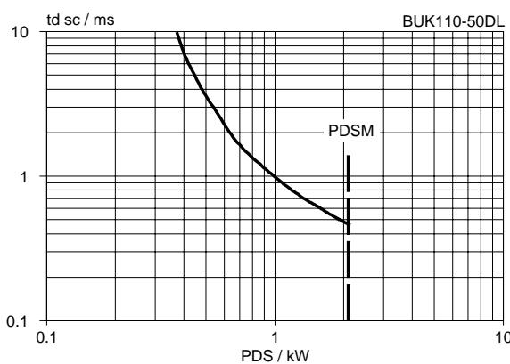
Fig.9. Typical overload protection characteristics.
