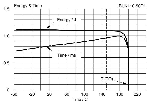
Fig.11. Typical overload protection characteristics.
