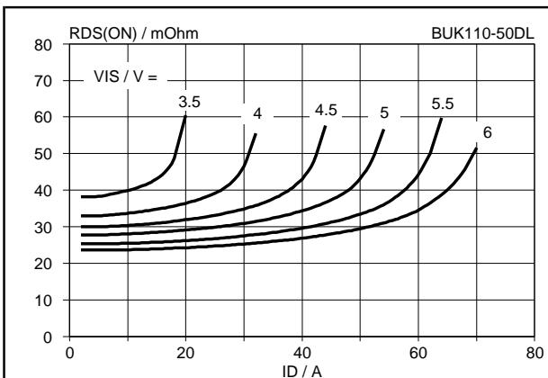
Fig.7. Typical on-state resistance,  $T_j = 25^\circ C$ .
