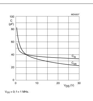
Fig.7 Input and output capacitance as functions of drain-source voltage, typical values per section.
