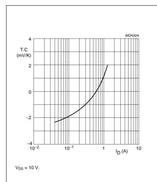
Fig.4 Temperature coefficient of gate-source voltage as a function of drain current, typical values per section.
