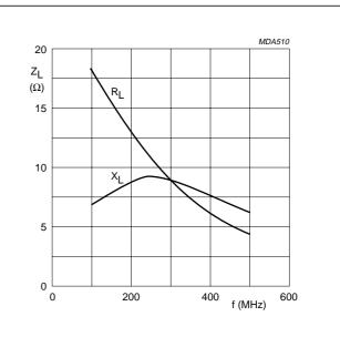
Class-B operation; V\_{DS} = 28 V; I\_{DQ} = 2 \times 40 mA; PL = 40 W.
