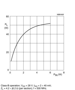
Fig.10 Load power as a function of input power, typical values per section.
