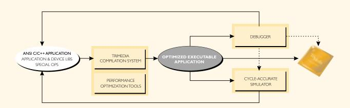
The TriMedia Software Development Environment includes a full suite of system software tools to compile and debug code, analyze and optimize performance, and simulate execution on TriMedia processors.
