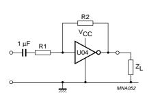
$Z_L > 10 \text{ k}\Omega$ ,  $R1 \ge 3 \text{ k}\Omega$  and  $R2 \le 1 \text{ M}\Omega$ .
