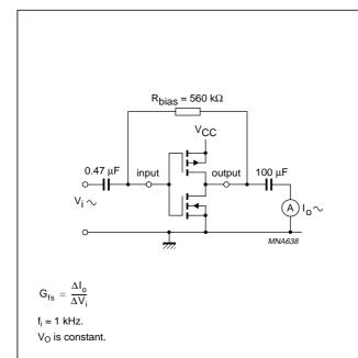
Fig.6 Test set-up for measuring forward transconductance.
