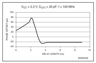
Figure 7. Phase offset vs. delay length
