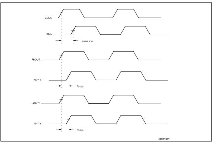
Figure 2. Phase Error and Skew Calculations
