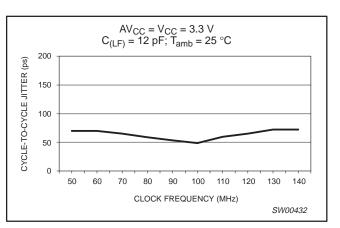
Figure 6. Cycle-to-cycle jitter vs. clock frequency
