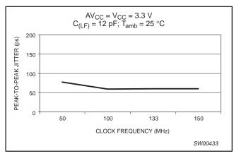
Figure 5. Peak-to-peak jitter vs. clock frequency
