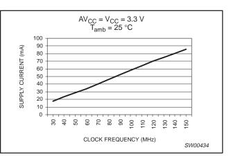
Figure 4. Supply current vs. clock frequency
