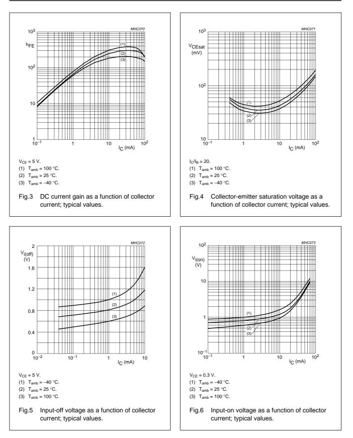
NPN resistor-equipped transistors; R1 = 10 k $\Omega$ , R2 = 47 k $\Omega$
