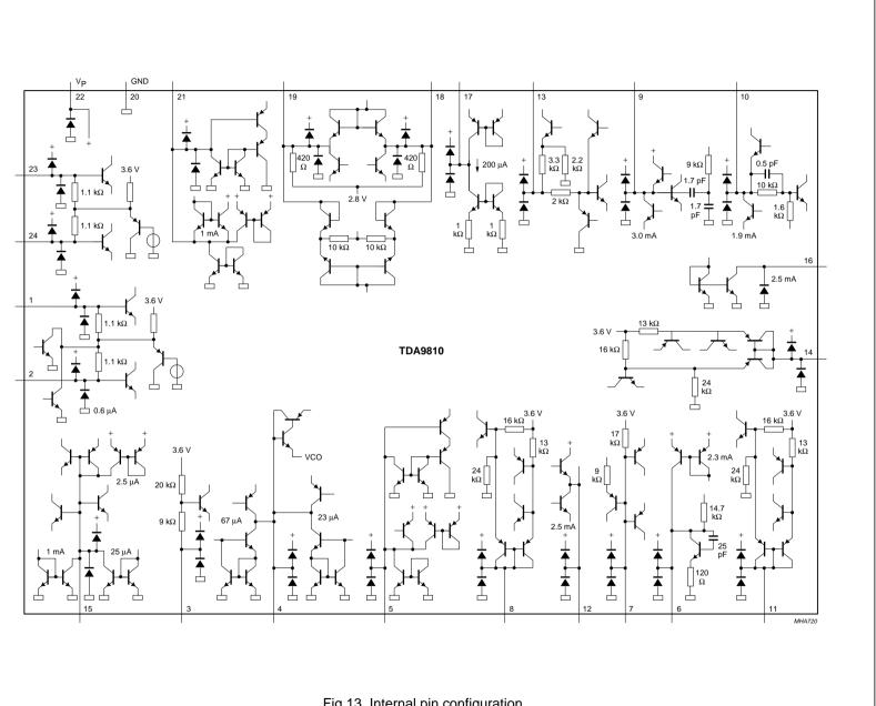
Fig.13 Internal pin configuration.
