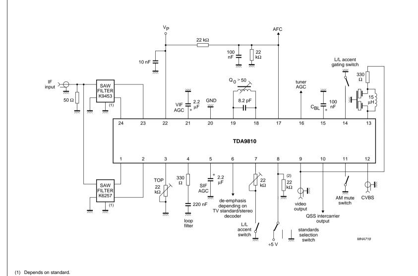
Fig.15 Application circuit.
