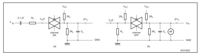
Figure 8. Test circuit for measuring crosstalk between any two switches. (a) channel ON condition; (b) channel OFF condition.
