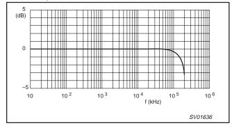
Figure 7. Typical frequency response.
