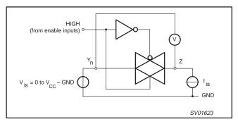
Figure 1. Test circuit for measuring ON-resistance ( $R_{ON}$ ).
