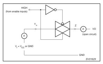
Figure 3. Test circuit for measuring ON-state current.
