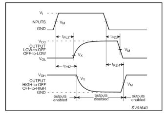
Figure 14. Turn-on and turn-off times for the inputs  $(S_n, \overline{E})$  to the output  $(V_{os})$ .
