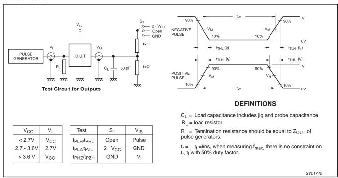
Figure 15. Load circuitry for switching times.
