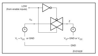
Figure 2. Test circuit for measuring OFF-state current.
