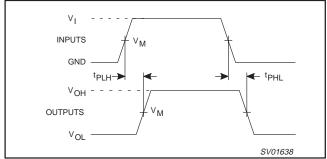
Figure 13. Input (V<sub>is</sub>) to output (V<sub>os</sub>) propagation delays.
