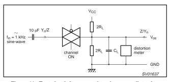
Figure 11. Test circuit for measuring sine-wave distortion.
