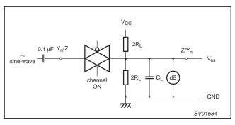
Figure 10. Test circuit for measuring minimum frequency response.
