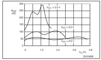
Figure 4. Typical ON-resistance (R<sub>ON</sub>) as a function of input voltage (V<sub>is</sub>) for V<sub>is</sub> = 0 to V<sub>CC</sub> – V<sub>EE</sub>.
