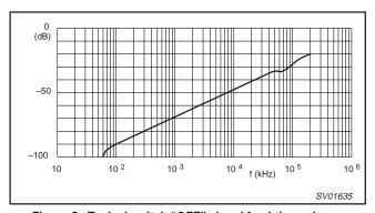
Figure 5. Typical switch "OFF" signal feed-through as a function of frequency.
