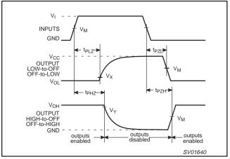
Figure 13. Turn-on and turn-off times for the inputs (nS,  $\overline{E}$ ) to the output (V<sub>os</sub>).
