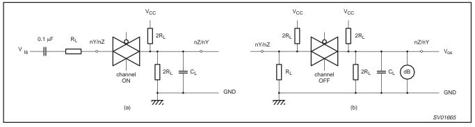
Figure 7. Test circuit for measuring crosstalk between any two switches.
