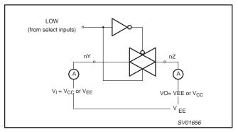
Figure 2. Test circuit for measuring OFF-state current.
