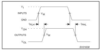
Figure 12. Input (Vis) to output (Vos) propagation delays.
