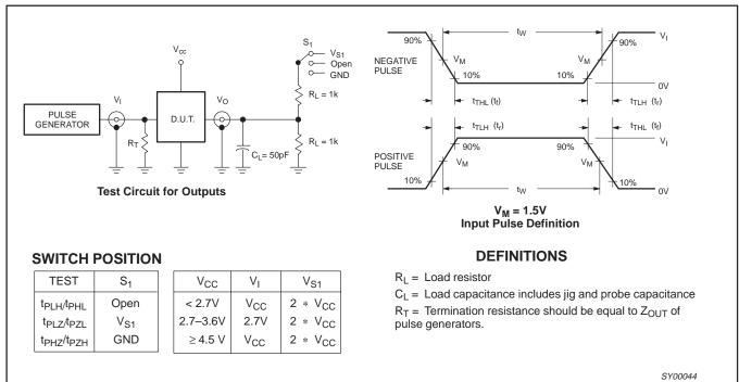
Figure 14. Load circuitry for switching times.
