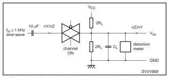
Figure 10. Test circuit for measuring sine-wave distortion.
