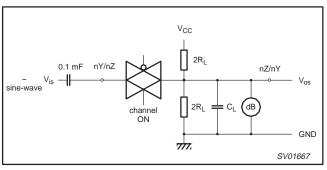
Figure 9. Test circuit for measuring minimum frequency response.
