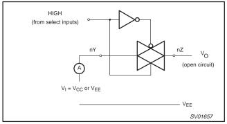
Figure 3. Test circuit for measuring ON-state current.
