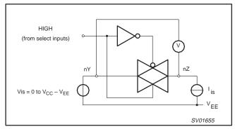
Figure 1. Test circuit for measuring ON-resistance (Ron).
