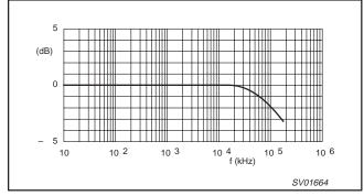
Figure 6. Typical frequency response.
