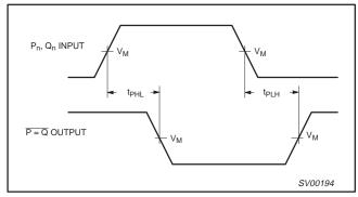
Propagation delays from the inputs  $(P_n, Q_n)$  to Waveform 2. the equal-to output  $(\overline{P} = \overline{Q})$ .
