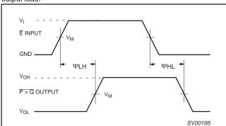
Propagation delays from the enable input (E) to Waveform 1. the equal-to output (P = Q).
