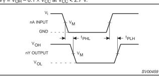
Figure 1. Input (nA) to output (nY) propagation delays.
