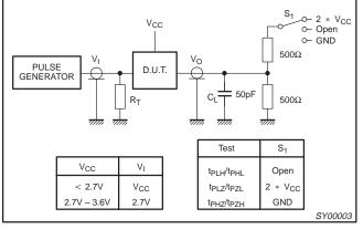
Figure 3. Load circuitry for switching times.
