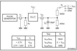
Figure 2. Load circuitry for switching times.
