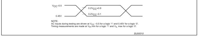
Figure 11. AC Testing Input/Output
