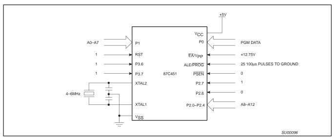
Figure 18. Programming Configuration
