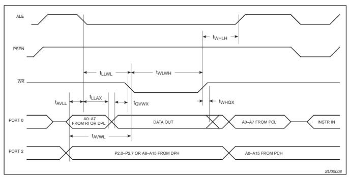
Figure 4. External Data Memory Write Cycle
