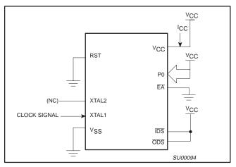
Figure 15. I<sub>CC</sub> Test Condition, Idle Mode All other pins are disconnected
