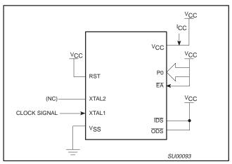
Figure 14. I<sub>CC</sub> Test Condition, Active Mode All other pins are disconnected
