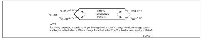
Figure 12. Float Waveform
