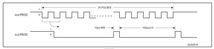
Figure 19. PROG Waveform
