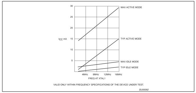
Figure 13. I<sub>CC</sub> vs. FREQ
