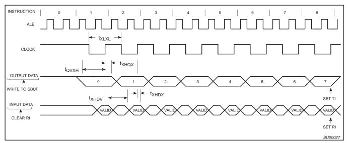
Figure 5. Shift Register Mode Timing
