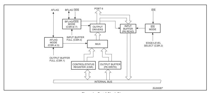
Figure 1. Port 6 Block Diagram
