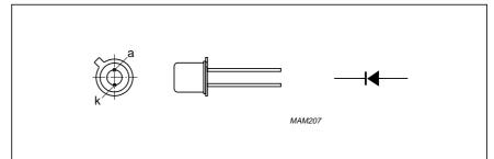
Fig.1 Simplified outline (SOT18/15; TO-18 except for the two leads) and symbol.
