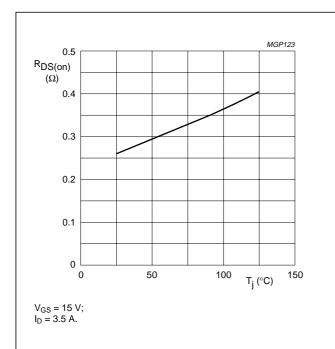
Fig.6 Drain-source on-state resistance as a function of junction temperature, typical values.
