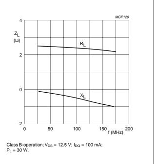
Fig.14 Load impedance as a function of frequency (series components), typical values.
