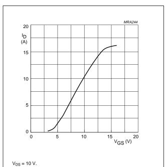
Fig.5 Drain current as a function of gate-source voltage, typical values.
