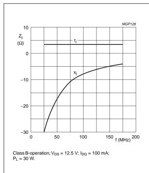
Fig.13 Input impedance as a function of frequency (series components), typical values.
