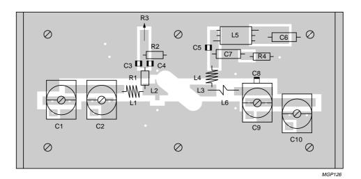
The circuit and components are situated on one side of the epoxy fibre-glass board, the other side being fully metallized to serve as earth. Earth connections are made by means of copper straps and hollow rivets for a direct contact between upper and lower sheets.
