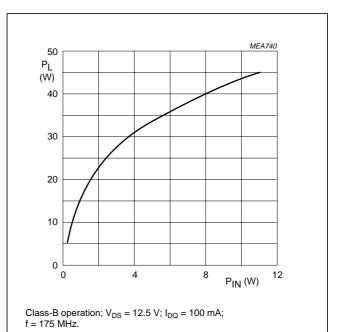
Fig.10 Load power as a function of input power, typical values.
