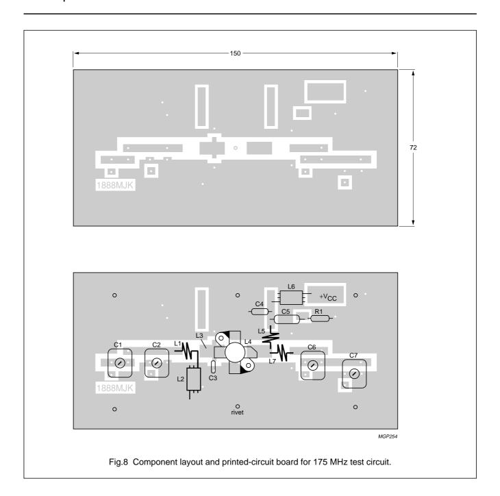
The circuit and the components are situated on one side of the epoxy fibre-glass board, the other side being fully metallized to serve as earth. Earth connections are made by means of hollow rivets, whilst under the emitter leads Cu straps are used for a direct contact between upper and lower sheets.
