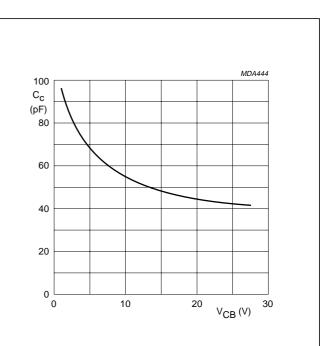
Fig.5 Output capacitance as a function of collector-base voltage; typical values.
