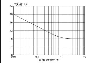
Fig.5. Maximum permissible repetitive rms on-state current  $I_{T(RMS)}$ , versus surge duration, for sinusoidal currents, f = 50 Hz;  $T_{mb} \le 111$  °C.
