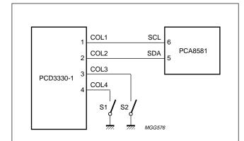
Fig.6 Circuit diagram for the EEPROM programming procedure.
