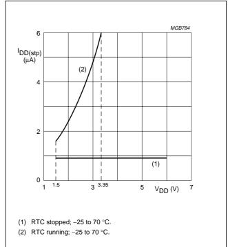
Fig.8 Typical supply current (I<sub>DD</sub>) in Stop mode as a function of supply voltage (V<sub>DD</sub>).
