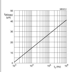
Fig.9 Typical supply current  $(I_{DD(stp)})$  in Stop mode as a function of counter frequency, both counters running in parallel.  $(V_{DD}=3~V;~T_{amb}=+25~^{\circ}C),$
