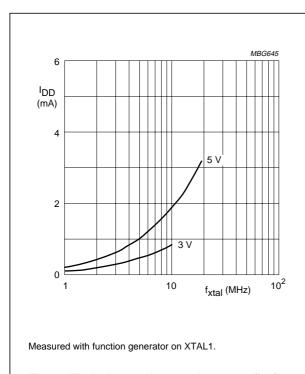
Fig.11 Typical operating supply current (I<sub>DD</sub>) as a function of clock frequency (fxtal).
