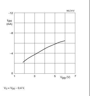
Fig.16 Typical HIGH level push-pull output source current ( $I_{OH}$ ) as a function of supply voltage ( $V_{DD}$ ).
