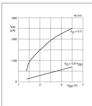
Fig.15 Typical HIGH level output pull-up source current ( $I_{OH}$ ) as a function of supply voltage ( $V_{DD}$ ).
