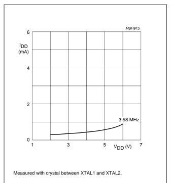
Fig.10 Typical operating supply current ( $I_{DD}$ ) as a function of supply voltage ( $V_{DD}$ ).
