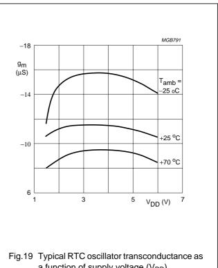
a function of supply voltage (V<sub>DD</sub>).
