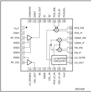
Figure 4. Pin-Out Block Diagram
