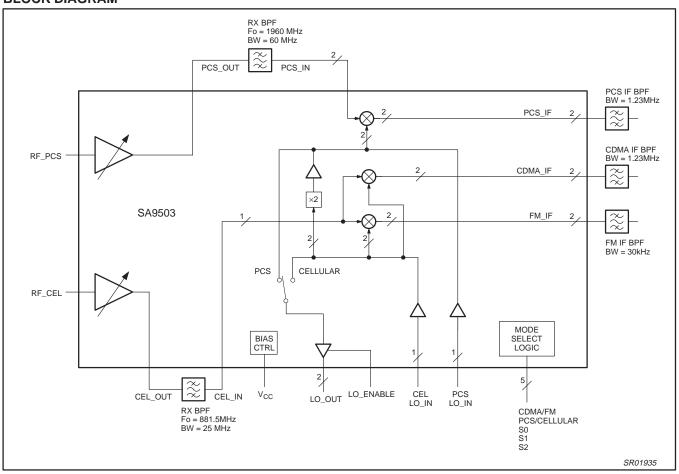
Figure 1. SA9503 Block Diagram
