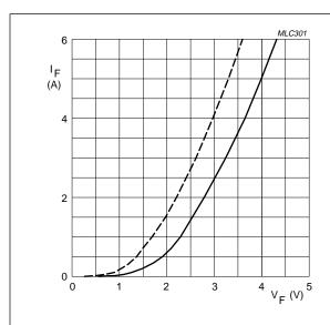
Dotted line:  $T_j = 175 \,^{\circ}\text{C}$ . Solid line:  $T_j = 25 \,^{\circ}\text{C}$ .
