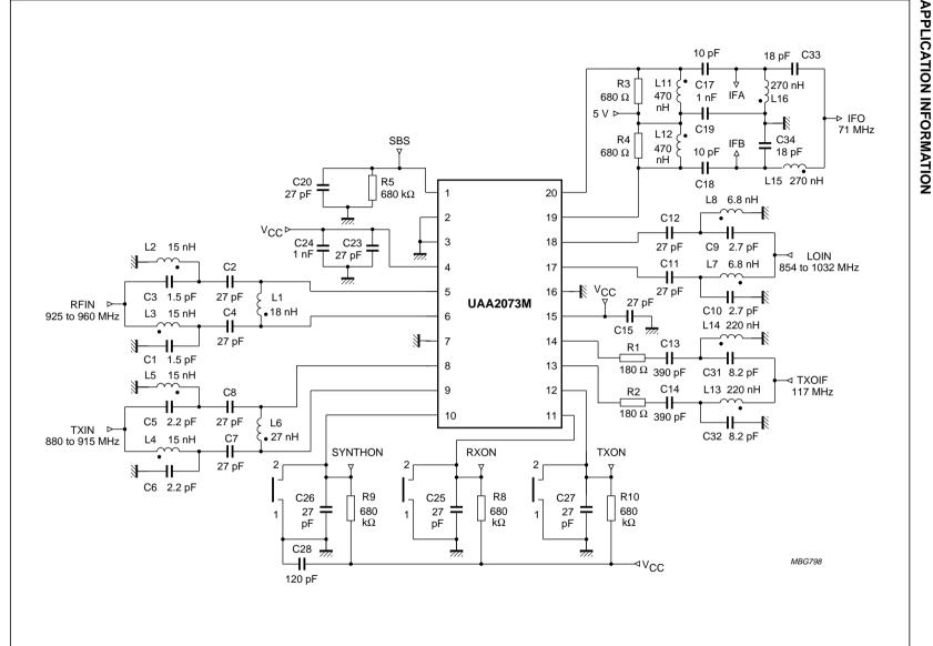
All matching is to 50  $\Omega$  for measurement purposes. Different values will be used in a real application.
