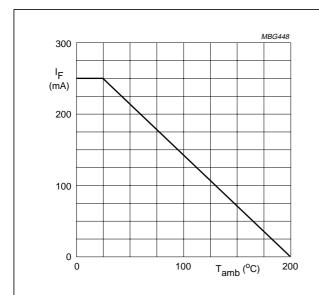
Device mounted on an FR4 printed-circuit board; lead length 10 mm.
