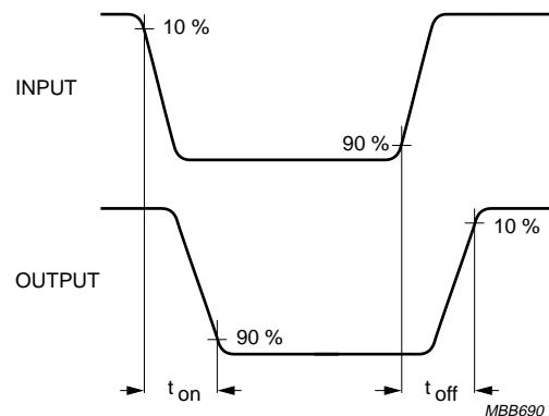
Fig.3 Input and output waveforms.
