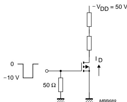
Fig.2 Switching time test circuit.
