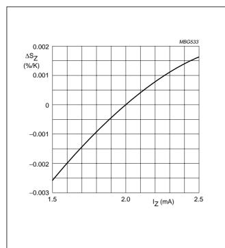
Fig.2 Temperature coefficient change as a function of working current; typical values.
