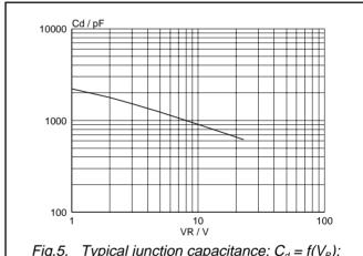
Typical junction capacitance;  $C_d = f(V_R)$ ; f = 1 MHz;  $T_j = 25$ °C to 125°C. Fig.5.
