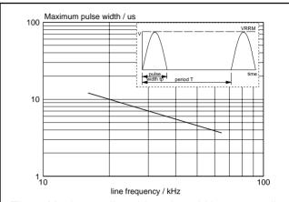
Fig.4. Maximum allowable pulse width  $t_p$  versus line frequency; Basic horizontal deflection circuit.
