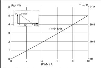
Fig.5. Total dissipation  $P_{tot} = f(I_{FWM})$ ; including forward recovery losses; Basic horizontal deflection circuit.
