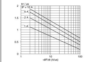
Fig.8. Maximum reverse recovery time  $t_{rr} = f(dl_F/dt)$ ; parameter  $T_j$ :  $V_R \ge 30V$
