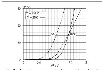
Fig.6. Typical and maximum forward characteristic  $I_F = f(V_F)$ ; parameter  $T_i$
