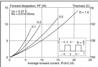
Fig.1. Maximum forward dissipation  $P_F = f(I_{F(AV)})$  per diode; square current waveform where  $I_{F(AV)} = I_{F(RMS)} x \sqrt{D}$ .
