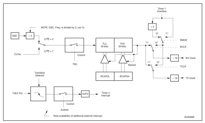
Figure 4. Timer 2 in Baud Rate Generator Mode
