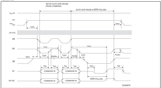
Figure 23. Automatic Chip Erase Timing Waveform
