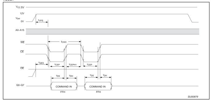
Figure 24. Reset Timing Waveform
