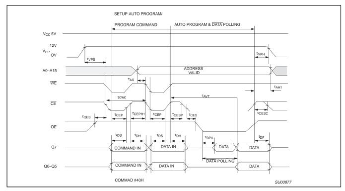
Figure 22. Automatic Programming Timing Waveform
