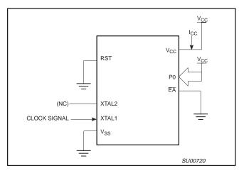
Figure 18. I<sub>CC</sub> Test Condition, Idle Mode All other pins are disconnected
