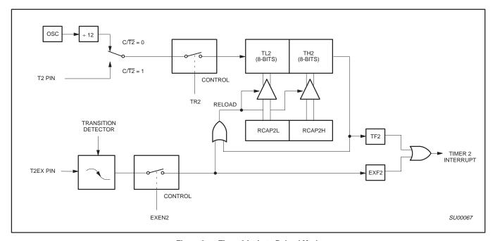
Figure 3. Timer 2 in Auto-Reload Mode
