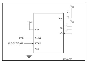
Figure 17. I<sub>CC</sub> Test Condition, Active Mode All other pins are disconnected
