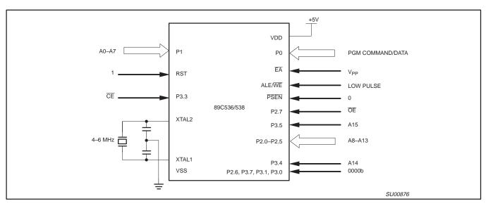
Figure 21. Erase/Programming/Verification
