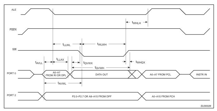
Figure 11. External Data Memory Write Cycle
