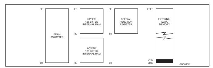
Figure 8. Internal and External Data Memory Address Space
