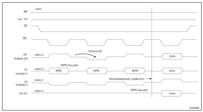
Figure 25. Toggle Bit, Data Polling Timing Waveform
