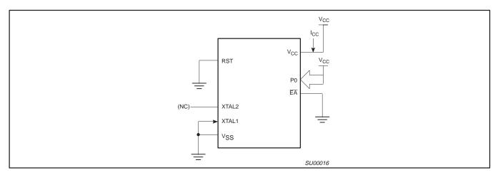
Figure 20.  $I_{CC}$  Test Condition, Power Down Mode All other pins are disconnected.  $V_{CC}$  = 2V to 5.5V
