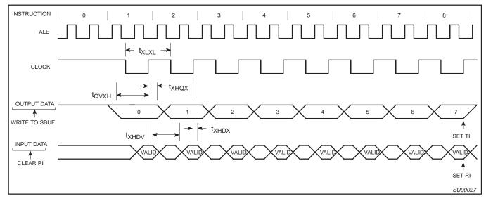
Figure 12. Shift Register Mode Timing
