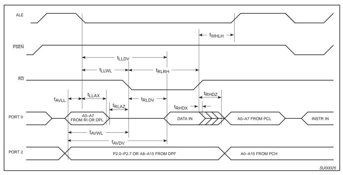
Figure 10. External Data Memory Read Cycle
