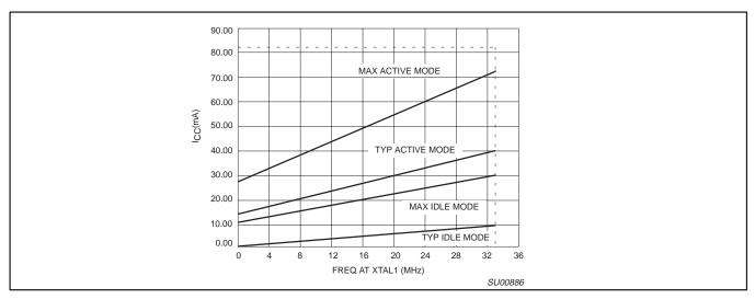
Figure 16. I<sub>CC</sub> vs. FREQ Valid only within frequency specifications of the device under test
