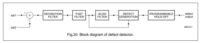
A defect detection circuit is incorporated into the SAA7370A. If a defect is detected, the radial and focus error signals may be zeroed, resulting in better playability. The defect detector can be switched off, applied only to focus control or applied to both focus and radial controls under software control (part of foc\_parm1).
