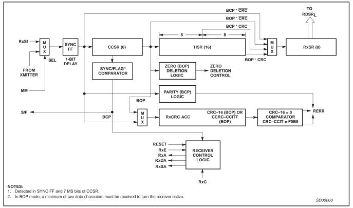
Figure 4. MPCC Receiver Data Path
