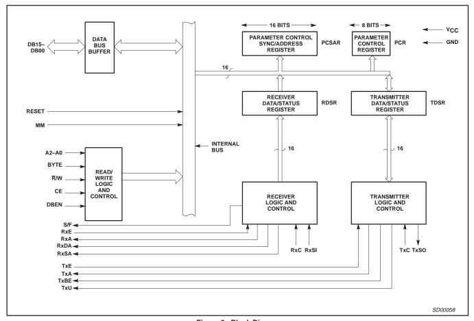
Figure 2. Block Diagram
