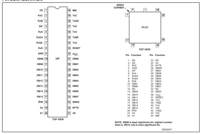
Figure 1. Pin Configuration
