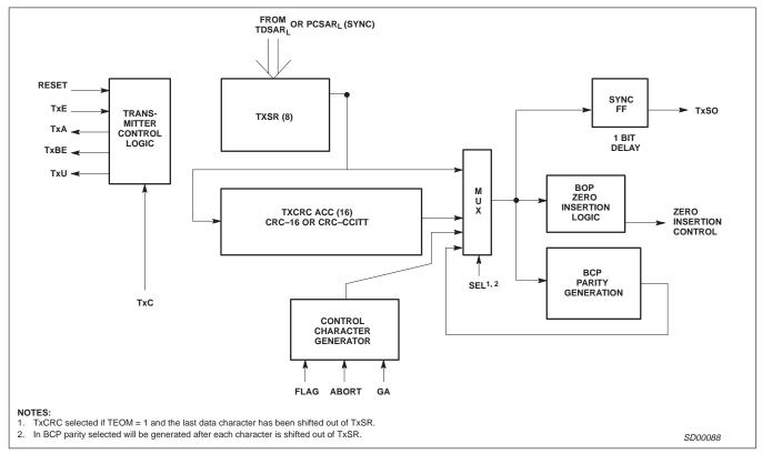
Figure 5. MPCC Transmitter Data Path
