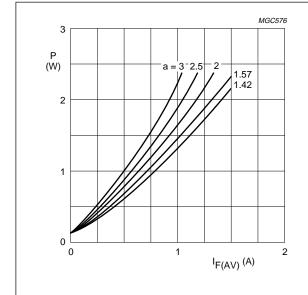
Fig.6 Maximum steady state power dissipation (forward plus leakage current losses, excluding switching losses) as a function of average forward current.
