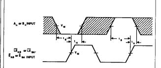
Waveform 4. Waveforms Showing the Data Setup and Hold Times for  $\mathbf{A}_{n}$  or  $\mathbf{B}_{p}$  input to Latch Enable ( $\overline{\mathsf{LE}}_{AB}$ ,  $\overline{\mathsf{LE}}_{BA}$ ) and Enable ( $\overline{\mathsf{E}}_{AB}$ ,  $\overline{\mathsf{E}}_{BA}$ ) inputs
