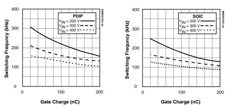
Figure 5. Switching Frequency versus Gate Charge for a) PDIP and b) SOIC.
