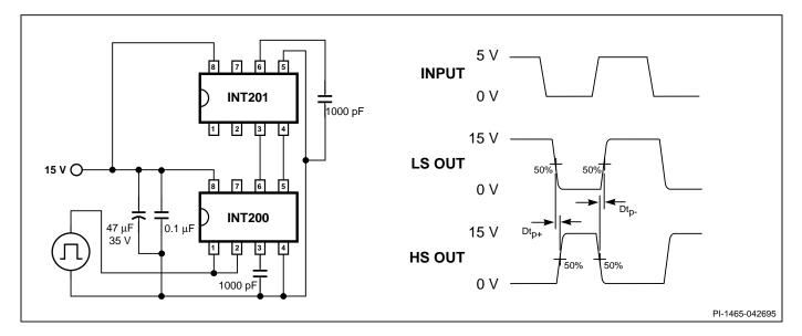
Figure 8. Dead Time Test Circuit.
