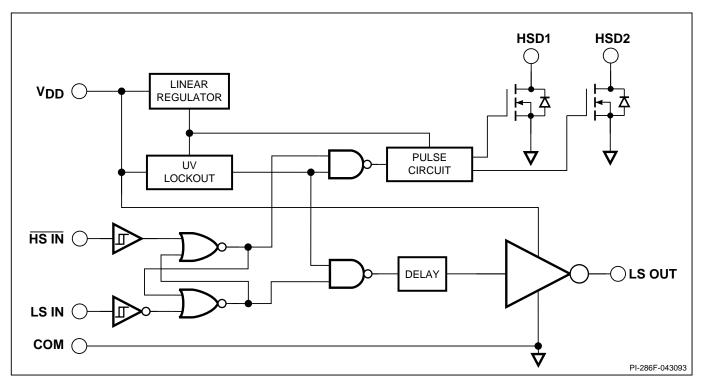
Figure 3. Functional Block Diagram of the INT200
