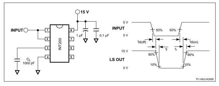
Figure 7. Switching Time Test Circuit.
