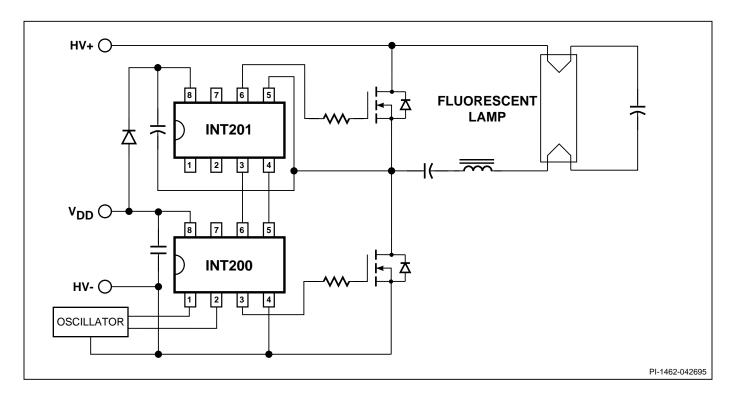
Figure 6. Using the INT200 and INT201 to Drive a Fluorescent Lamp.
