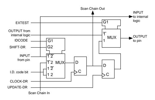
Figure 10: Layout of Output Enable and Bidirectional Cells
