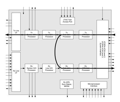
Figure 20: Data Diagnostic Loopback Mode
