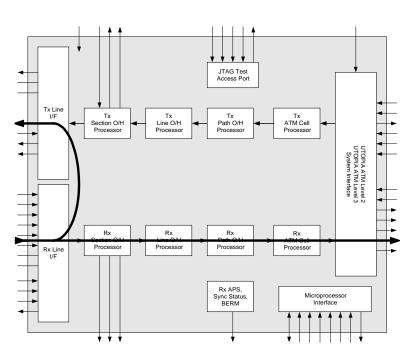
Figure 16: Line Loopback Mode
