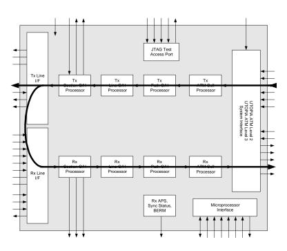
Figure 18: Parallel Diagnostic Loopback Mode
