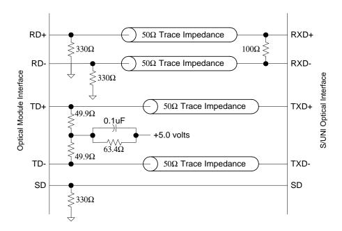
When a PECL input is not being used, the positive differential input must be tied to analog power (AVD) and the negative differential input must be tied to analog ground (AVS). In all cases, the PECL inputs must be driven with a differential voltage (do not connect both pins to AVD or AVS).
