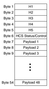
Bit 7 of each byte is the most significant bit (which corresponds to the first bit transmitted or received). The header check sequence octet (HCS) is passed through this structure. The start of cell indication input and output (TSOC and RSOC) are coincident with Byte 1.
