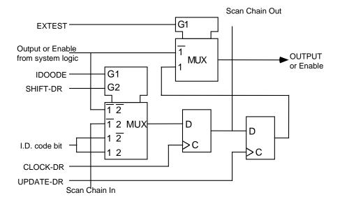
Figure 9: Bidirectional Cell (IO\_CELL)
