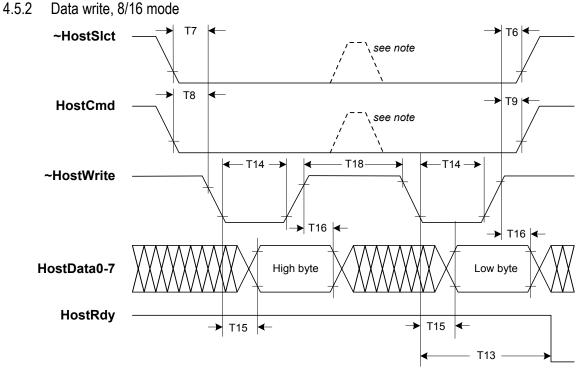
Note: If setup and hold times are met, ~HostSlct and HostCmd may be de-asserted at this point.
