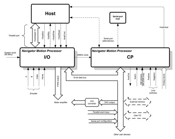
The CP chip contains the profile generator, which calculates velocity, acceleration, and position values for a trajectory; and the commutation unit, which calculates a motor command for each motor phase. The commutation unit produces one of two types of output:
