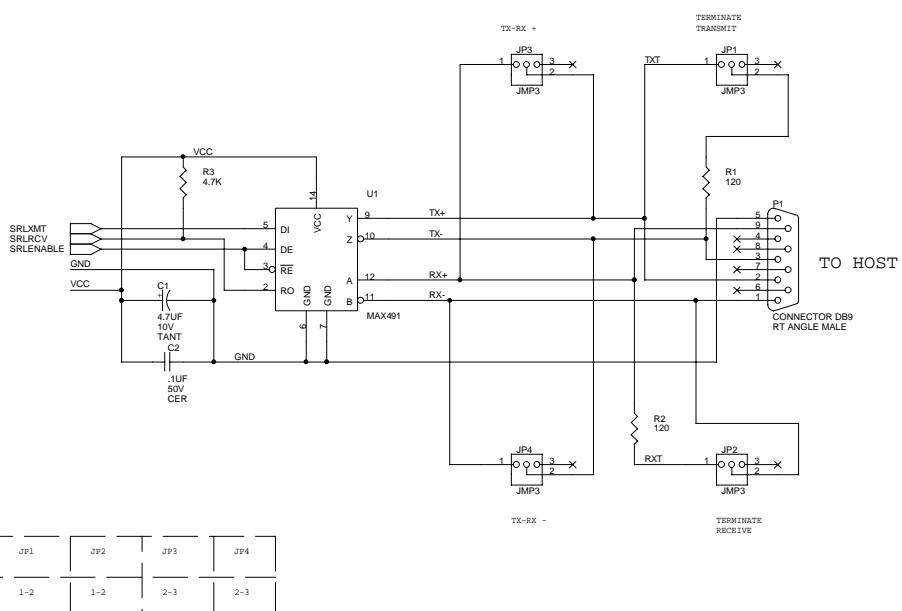
NOTE:RS422 IS CAPABLE OF FULL DUPLEX AND USES 2 PAIRS.
