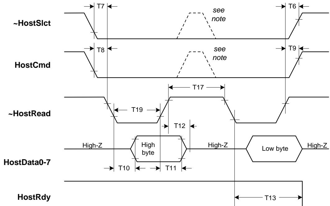
Note: If setup and hold times are met, **~HostSlect** and **HostCmd** may be de-asserted at this point.
