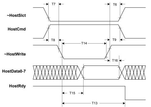
4.4.2 Data write, 8/8 mode Τ7 see note ~HostSlct Т8 ┥ see note HostCmd T18 -T14 → - T14 -4 ┢ ◄ ~HostWrite ► T16 🔫 HostData0-7 High byte Low byte
