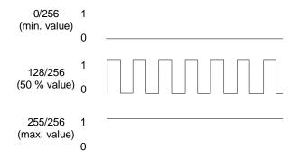
An output pulse width of 0 parts per 256 represents the minimum voltage, an output pulse width of 128 per 256 (50 %) represents a voltage of 50 % total scale and a pulse width of 256 per 256 represents the maximum positive voltage.
