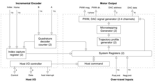
The above figure shows an internal block diagram for the MC1241A motion processor.
