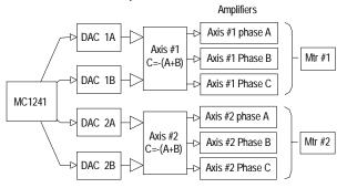
When using DAC output mode the digital word provided by the chipset must first be converted into a voltage using an external DAC. Two DAC channels are required per axis. The third phase is constructed externally using the expression C = -(A+B). This is usually accomplished with an Op-amp circuit.
