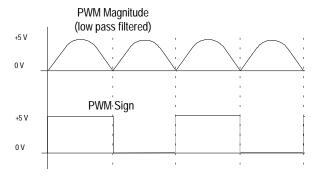
In this diagram the PWM magnitude signal has been filtered to convert it from a digital variable duty cycle waveform to an analog signal.
