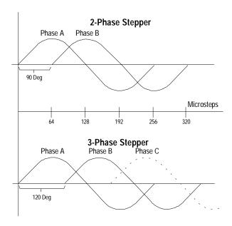
For 3-phase stepper motors or AC Induction motors, the phase C waveform must be constructed externally using the expression C = - (A+B). Typically this is performed by the motor amplifier itself. See the following section of this manual entitled "Motor Output" for more information.
