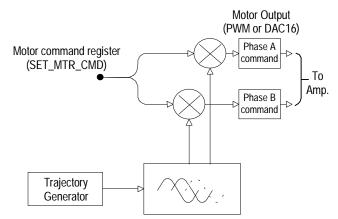
The microstepping portion of the chipset generates a sinusoidal waveform with 64 distinct output values per full step (one full step = a quarter electrical cycle).
