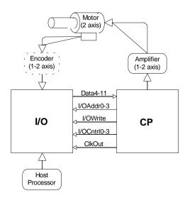
The CP and I/O chips function together as one integrated motion processor. The major components connected to the chip set are the optional encoder (2, or 1 axes), the motor amplifier (2, or 1 axes), and the host processor.
