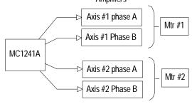
Using the DAC output mode the digital motor output word for each phase is typically converted into a DC signal with a value between -10 to +10 volts. This signal can then be input into an off-the-shelf DC-Servo type amplifier (one amplifier for each phase) or into any other linear or switching amplifier that performs current control and provides a bipolar, two-lead output.
