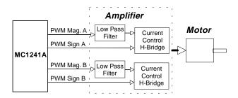
Relative to the DAC output method the PWM output mode when used with this amplifier scheme has the advantage of high performance with a minimum of external parts. This amplifier scheme is shown below for a single motor axis (two phases).
