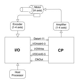
The CP and I/O chips function together as one integrated motion processor. The major components connected to the chip set are the Encoder (4, 2, or 1 axes), the motor amplifier (4, 2, or 1 axes), and the host processor.
