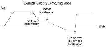
There are no restrictions on switching the profile mode to velocity contouring while the axis is in motion.
