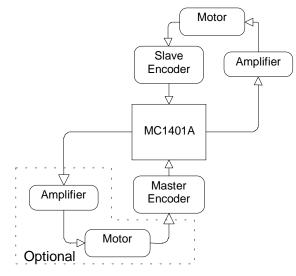
Because a geared axis takes up two encoder channels, the total number of geared axes supported per chipset is 1/2 the total # of axes.
