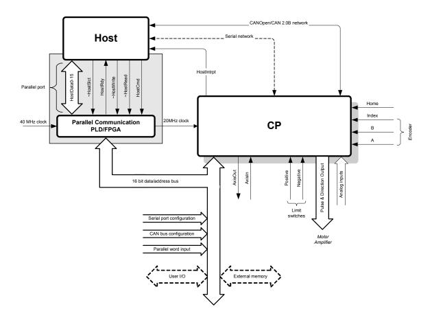
The shaded area shows the CPLD/FPGA that must be provided by the designer if parallel communication is required. A description and the necessary logic (in the form of schematics) of this device are detailed in section Parallel FPGA of this manual.
