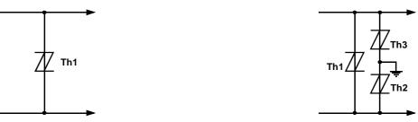
Figure 12. TWO POINT PROTECTION
