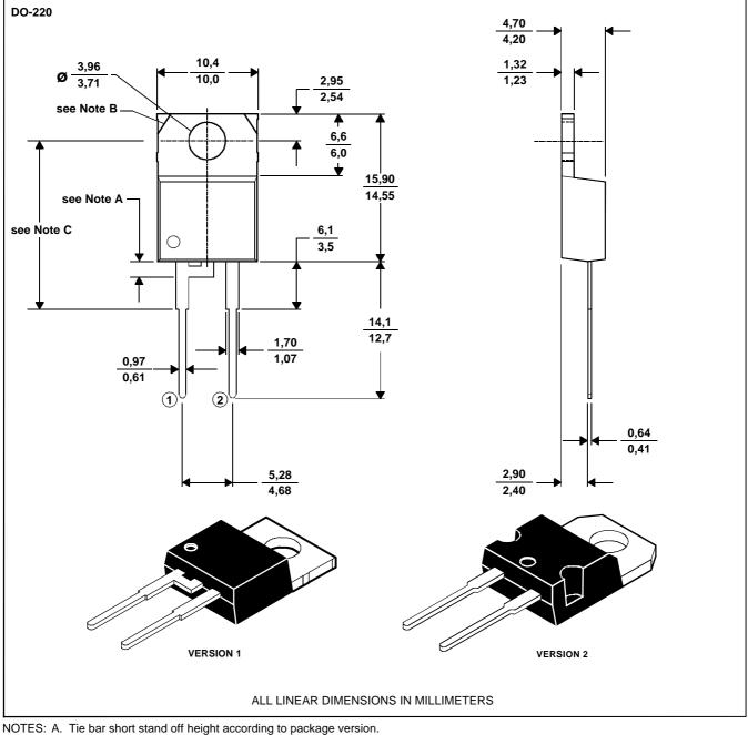
Version 1, pin 1 is in electrical contact with the mounting tab via tie bar short - stand off height : 2,0 mm maximum.
