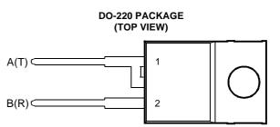
Pin 1 is in electrical contact with the mounting base.
