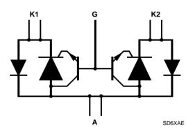
Terminals K1, K2 and A correspond to the alternative line designators of T, R and G or A, B and C. The negative protection voltage is controlled by the voltage,  $V_{\text{GG}}$ , applied to the G terminal.
