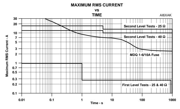
Figure 8. '1089 MAXIMUM TEST CURRENT LEVEL
