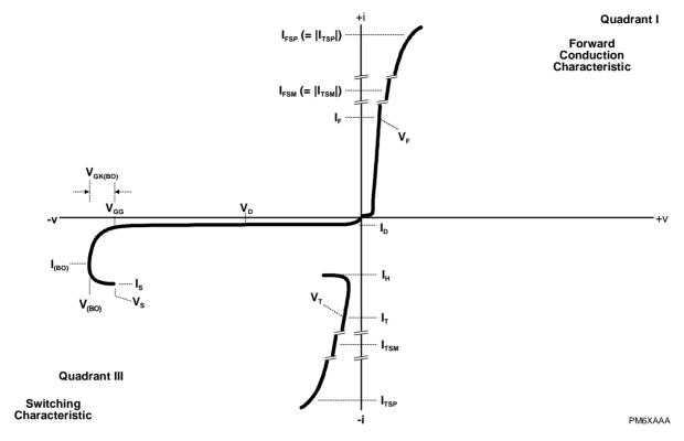
Figure 1. VOLTAGE-CURRENT CHARACTERISTIC
