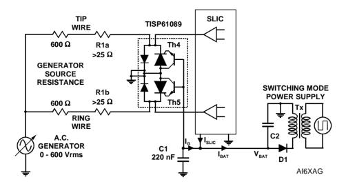
Figure 3. TISP61089 BUFFERED GATE PROTECTOR (SECTION 4.5.12 TESTING CONDITION)
