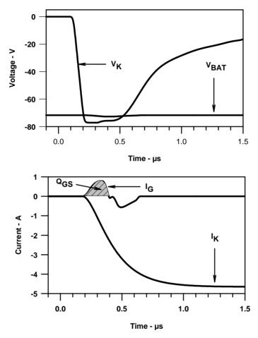
Figure 6. PROTECTOR FAST IMPULSE CLAMPING AND SWITCHING WAVEFORMS
